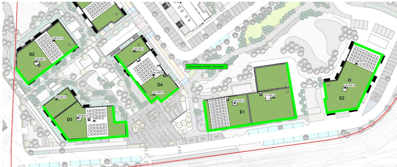
Figure 8.10 Facades requiring acoustically rated windows.
